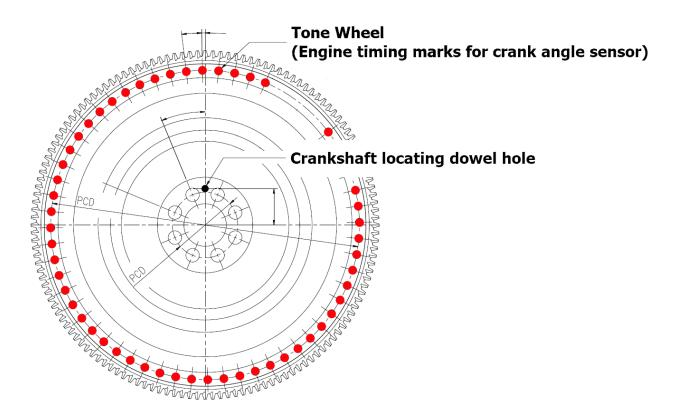
**Note:** The design, number of timing marks and the location of timing marks can differ depending on the vehicle application and/or engine specifications (even within the same model vehicle). The positioning of timing marks for this replacement flywheel (in relation to the crankshaft locating dowel) need be checked alongside the old item prior to installation in order to prevent fitment of incorrect parts.
