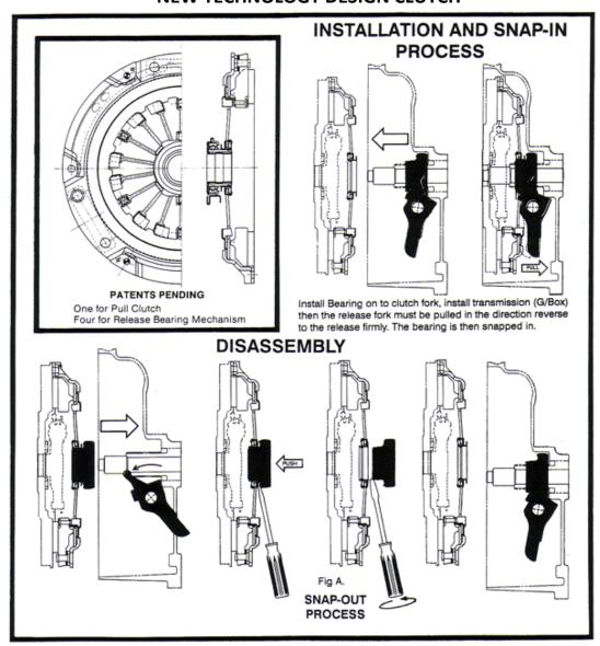
Procedure: move bell-housing back approximately 30 to 40mm, insert screwdriver and twist as Figure A. Bearing will then snap out from its retaining clip.
