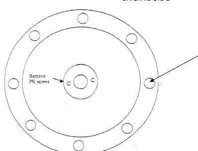
Drill head of all aluminum rivets using ½ inch drill to allow the ring gear to fall off. Drill rivets off the back of the ring gear and fit to new flywheel by the heat shrink method.
