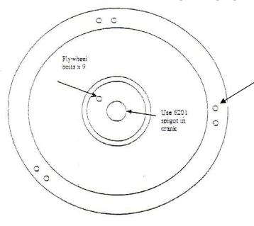
Remove & relocate dowels from dual mass flywheel to the new flywheel.
