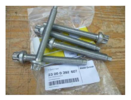
The engine block and gearbox housing on the models above are made from a light alloy metal. The gearbox housing is attached to the engine block using aluminium bolts. These aluminium bolts prevent electrochemical corrosion and must be replaced with new bolts every time the housing is removed from the engine block.
