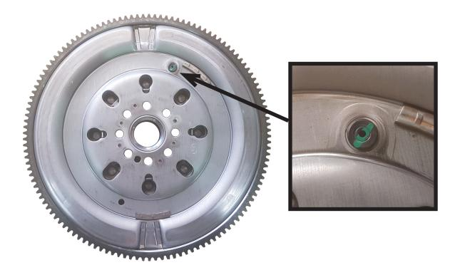
The Dual Mass Flywheel in this kit may be fitted with a transport fastener which contains a detent pin (see image above). This pin stops the two masses from moving against each other before the engine is started for the first time after installation.
