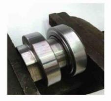
Using a vice, press the release bearing onto the carrier. Ensure correct orientation of the bearing, i.e. bearing contact surface with radius should face away from carrier.
