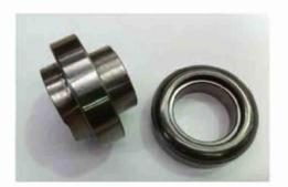
Release bearing and carrier as supplied in this clutch kit.
