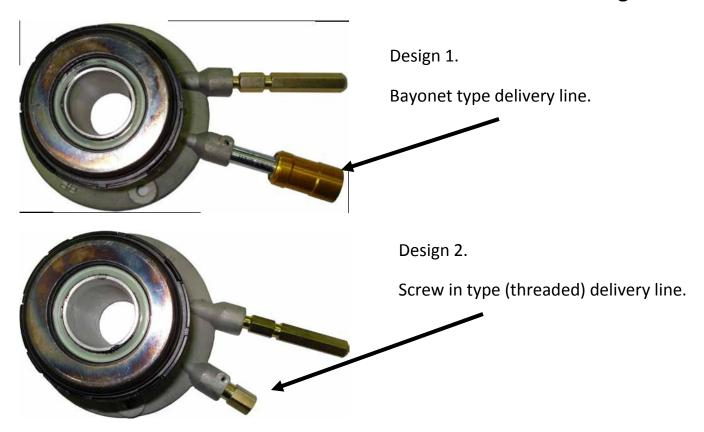
Should you encounter a vehicle with an incorrect delivery line fitting, both line fittings are interchangeable & can be removed by removing the roll pin using a suitable pin punch.
